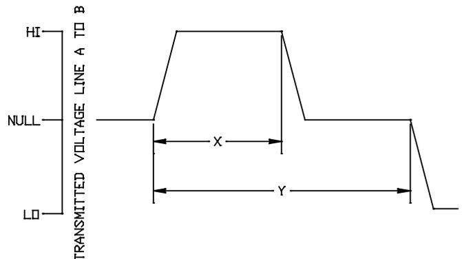
**Figure 2** Slew Rates and Bit Timing Diagram
