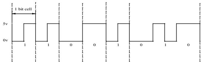
Figure 10 Harvard Bi-phase Bit Encoding
