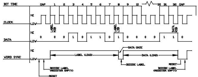
Figure 9 ARINC 561 6-Wire Bit Encoding
